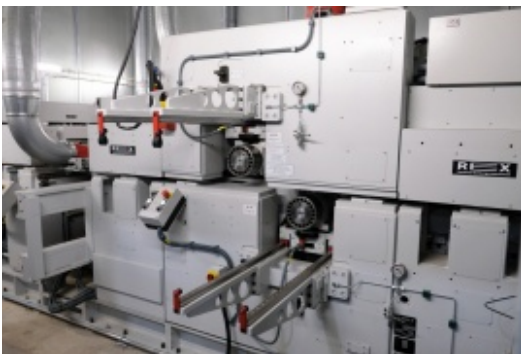
With Rex's Supermaster HC lamination planer, van Roje wants to save 1.5 mm of wood per lamination © Günther Jauk
